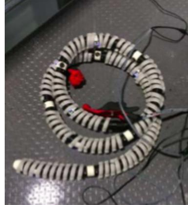
Fig. 1 Hose-shaped rescue robot.
